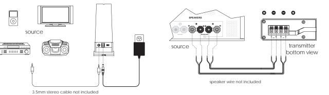
be sure to also plug-in the power supply as shown in option a
